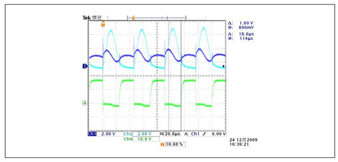
Figure 2-4 Waveform of the Synchronization Circuit
